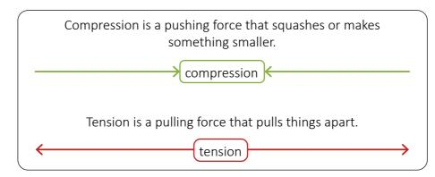
When these forces are balanced, a bridge is strong and stable. When they are unbalanced, a bridge will collapse.
