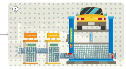
When the in valve is opened, the air under high pressure moves into the actuator and forces the piston to rise, lifting the car up. The air is released through the out valve to lower the piston back down again.
